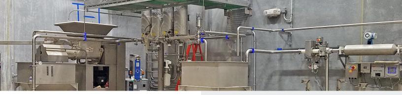
product from ~102F to ~32F. Based on the product mix and density, Williams-Carver provides the proper quantity of Votators based upon max product flow in lbs./hour to meet that cooling rate.
