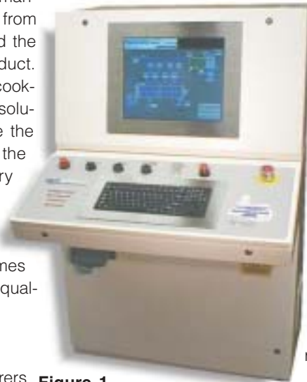
Figure 1. Extrusion control system console. Once thought to be too expensive and unreliable, cooking extrusion automation is now one of the most effective means for improving process efficiency.
