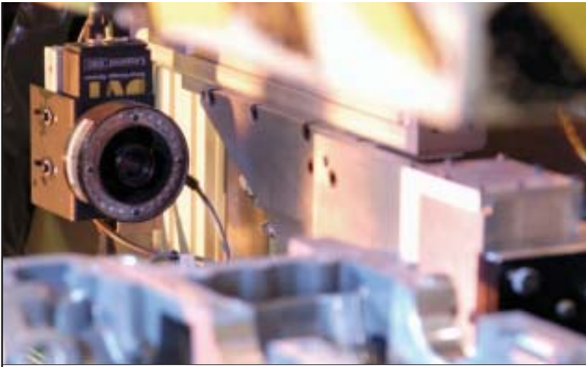
DVT's SmartImage Camera inspects bearings, balance shafts and snap ring seating in the engine transmission block of the Harley-Davidson V-Rod motorcycle.
