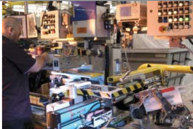
A DVT Legend SmartImage 530 camera, tied in to an Allen-Bradley PLC, provides a 100 percent inspection rate for bearing and balance shaft presence and proper snap ring seating in Harley-Davidson V-Rod engine transmission blocks.
